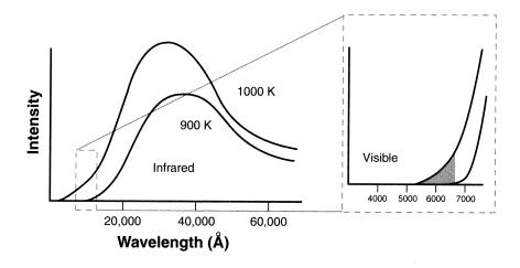
When you heat up an object, the peak of its radiation starts way out in the infrared. As you heat it up more, the peak moves to shorter and shorter infrared wavelengths—that is, it moves closer to the red. At this temperature, you see the toaster (or a star being born) glowing reddish. As it heats up more, it gives off more energy in the red, though the peak of the radiation is still out in the infrared. When it gets hot enough,
