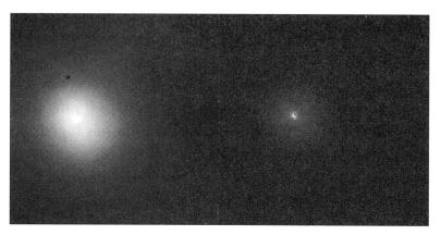
When the adaptive optics system was turned on at the Keck 2 telescope, to counteract the effects of seeing by distorting one of the telescope's mirrors, the image size improved by a factor of over 10. This infrared image of a star improved from the blurry half an arc second (left) to the more pinpoint ½0 of an arc second (right); both images are shown to the same scale.
