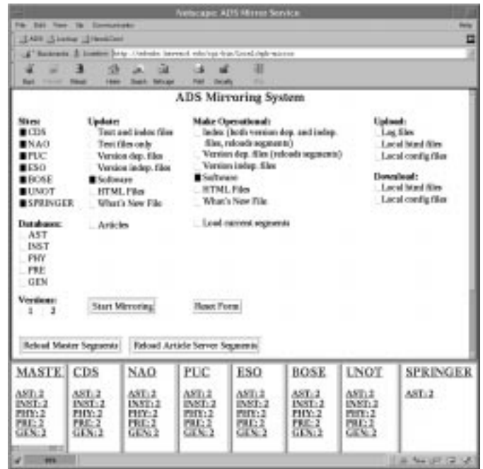
Fig. 7. The WWW interface used by the ADS administrators to update different components of the databases on the different mirror sites. The small windows at the bottom of the screen display, for each of the ADS databases, the version number currently operational at each mirror site
